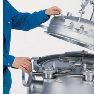
3 Opening the cover aided by spring assisted mechanism
